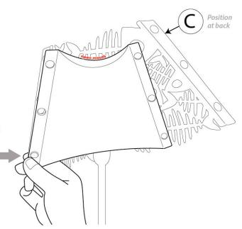
7) Holding the top button area, slide up via the gap.
