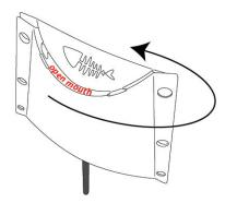
6) Hold the Fish Bone shade at the back and align the 3 holes in position
